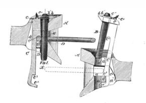
of C. M. Hoag. of Greenbush, an engineer on the Boston and Albany Railroad. At the trial it was the only one that made the "flying switch" automatically. In its normal condition the link is level, and works successfully on all cars. The recommendations of the
