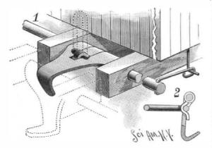
any special finish; it requires but one hand of the train man to operate it, and it adjusts itself automatically to the vertical and lateral movements of the car.
